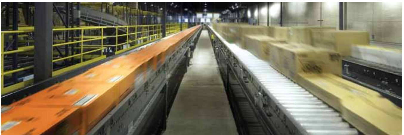
Conveyor systems can move product quickly and efficiently through a warehouse or distribution center. The speed of handling depends on the product being conveyed.
